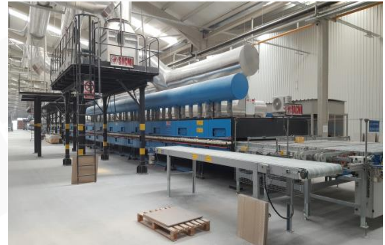
Above: Kiln exit with electricity co-generation Below: Laser-guided robotic forklifts
